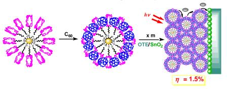
composite electrode reaches as high as 1.5%, which is 45 times higher than that of the reference system consisting of the both single components of porphyrin and fullerene.
